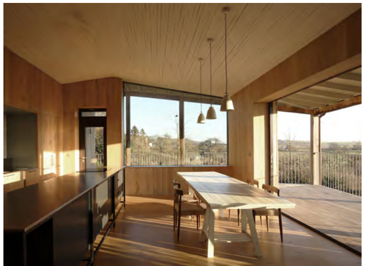
Fig.8.9 - Overhanging roof works in harmony with the energy strategy of this passivhaus by providing summer shading to the large areas of glazing positioned to the south-east. (Dundon Passivhaus by Prewett Bizley Architects ) [Credit: Passivhaus Trust / Prewett Bizley Architects]
