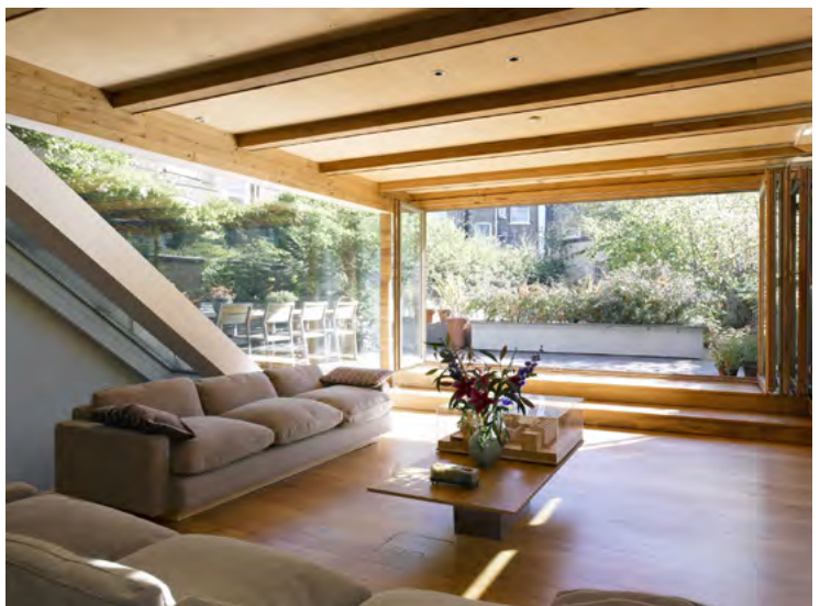
Fig.5.23 - Large areas of glazing to the living space control views to avoid overlooking or being overlooked.
