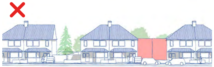
Fig.5.9 - Maintaining rhythm Conjoining buildings can create long street frontages and have a negative impact on the character of the street.
