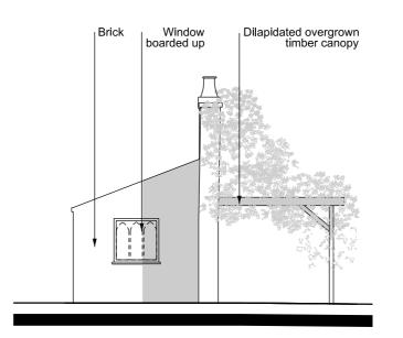
West Elevation Existing Drawings Potting Shed 0024 1:100@A3
