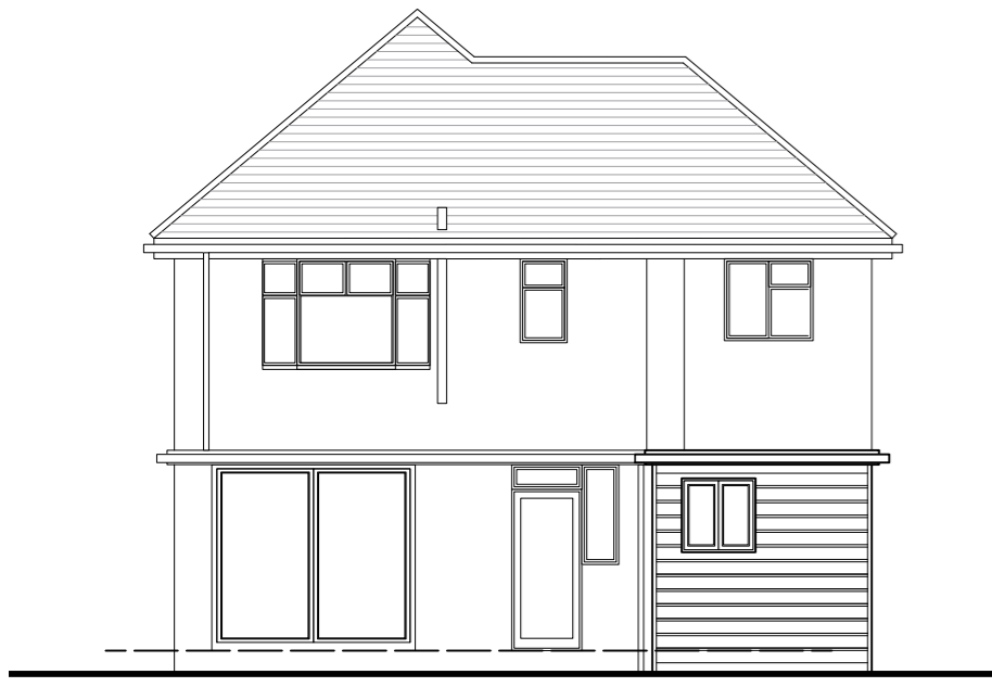
Dining Room Utility West Elevation [Rear] 1:100
