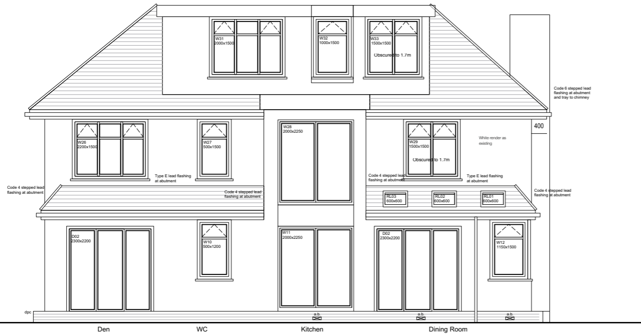
West Elevation [Rear] 1:50
