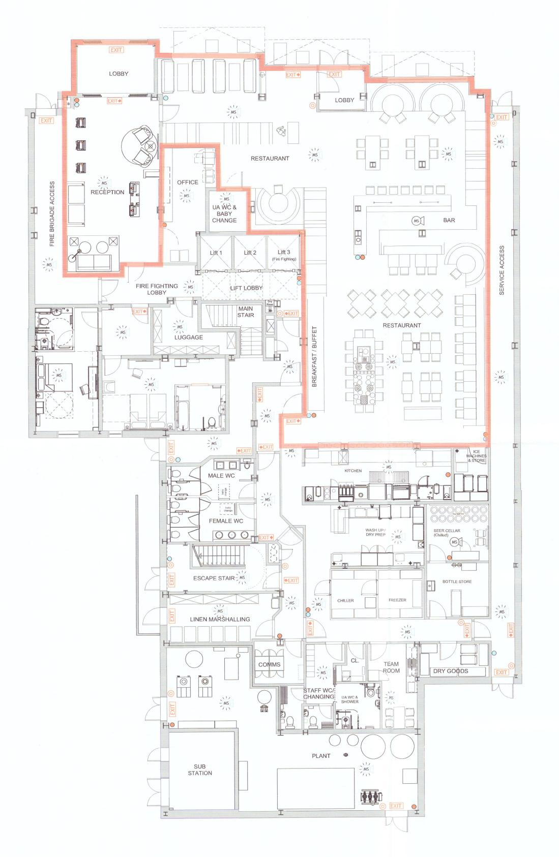
LICENSING SYMBOL KEY 6kg Powder Fire Extinguisher 2kg CO<sup>2</sup> Fire Extinguisher 6lt AFFF foam Fire Extinguisher Illuminated Exit Sign Illuminated Directional Sign - Straight Ahead Illuminated Directional Sign - Left / Right Combined multi-criteria sensor/sounder/beacon Combined multi-criteria sensor & sounder Fire alarm call point
